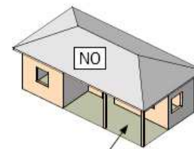
Veranda too deep
