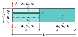
Fig. 6: The asymmetric double cantilever beam (ADCB) test
