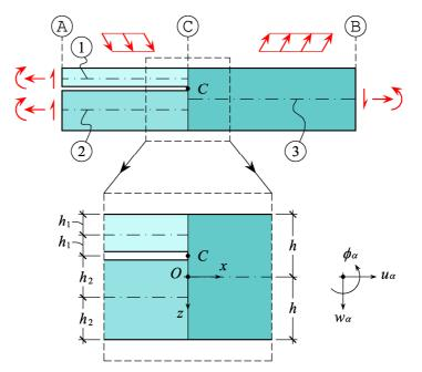
Fig. 2: The delaminated laminate as an assemblage of three laminated beams
