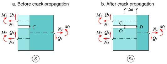
Fig. 3: Elementary segment of the laminate in the neighbourhood of the crack tip
