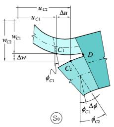
Fig. 4: Crack-tip relative displacements in system S<sub>0</sub>
