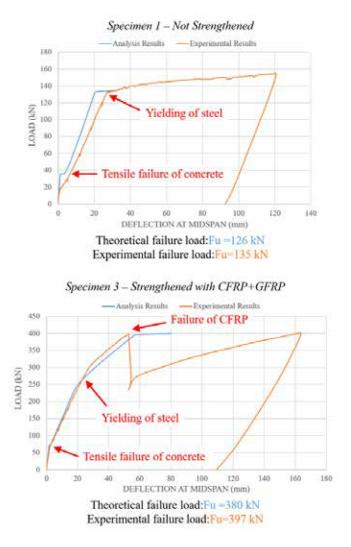
Figure 5 - Comparison between the theoretical and experimental load-deflection curves
