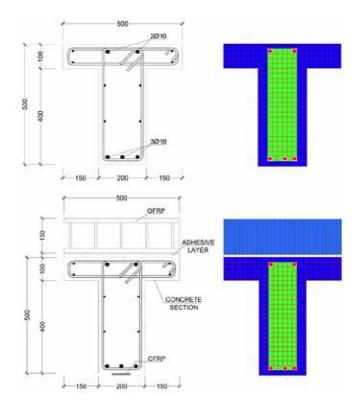
Figure 4 - Cross sections and finite element models of the prototype beams (specimens 1 and 3)
