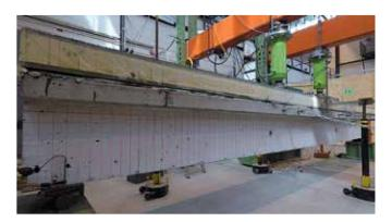
Figure 3 - Prototype beam strengthened with the SUREBridge technique and tested in the laboratory
